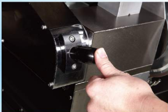
Locking Device for Grinding Wheel Dismantling 拆卸砂輪的剎車裝置
